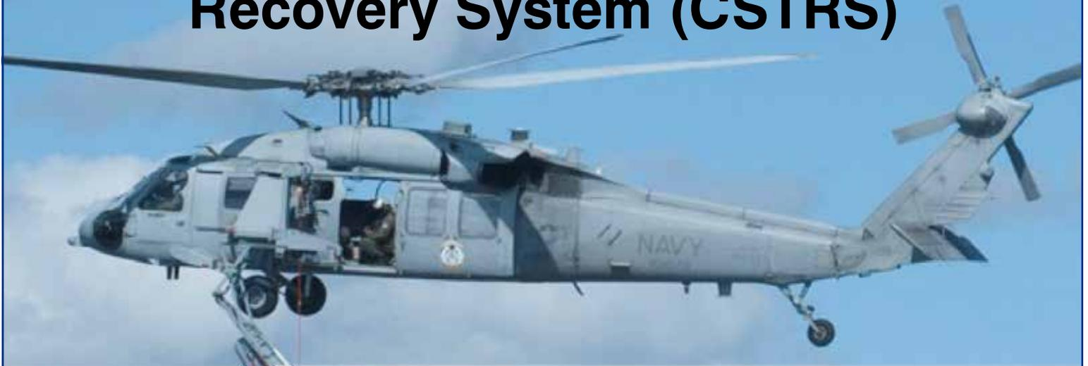
The Carriage, Stream, Tow, and Recovery System (CSTRS) is a launch and handling system that was designed to support the U.S. Navy's requirement to provide an organic airborne mine countermeasure capability from an H-60 helicopter. CSTRS enables rapid response to mine threats, providing an extra measure of safety for crew and ships during shallow water missions. In addition, the CSTRS design is modular and is capable of supporting the deployment
