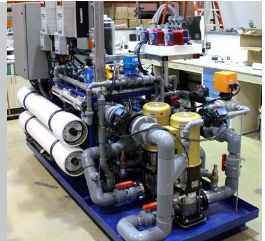
Twin Ultra 10,000 gal/day (38m³/day) skid-mounted, water recycling system
