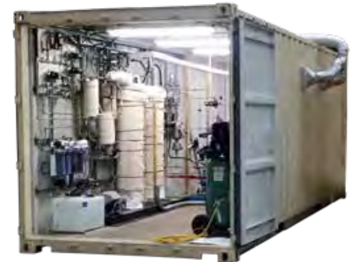
Generating hydrogen fuel through on-site waste conversion potentially eliminates the need to transport fuel/energy sources to the field.
