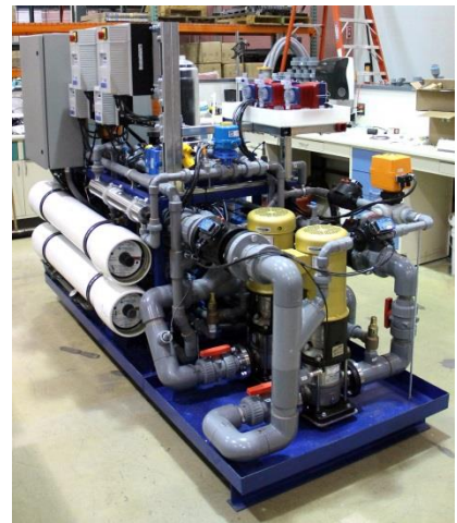
Enterprise Ventures Corporation's Twin Ultra Greywater Recycling System can be custom designed to recycle 60 to 90% of greywater at a rate up to 10,000 gallons per day.
